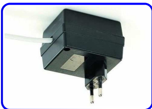
1. External power supply (input 220-240 VAC; output 5 VDC; 200 mA )
